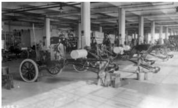
Model T chassis at Ford Motor Company plant, Highland Park, Michigan, about 1910
