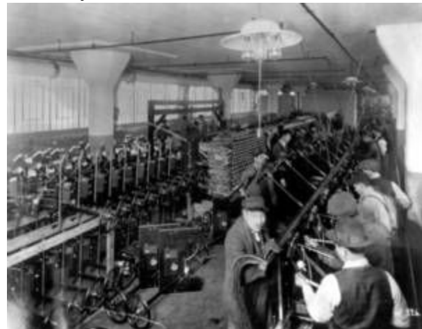
Workers assembling Model T dashboards at Ford Motor Company plant, Highland Park, Michigan, about 1913
